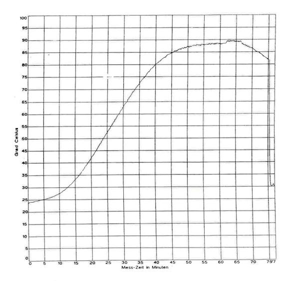
Note: Disturbance at 62 minutes seen on curve is due to the transfer of the disinfection container from the warming unit to the cooling unit
